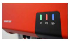
For many inverters, all three LED lights will come on and stay solid for a period of time upon start-up. It may take up to 10 minutes for the inverter to finish turning all the way back on.
